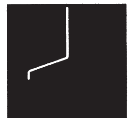
B-E paralleled by 680Ω
