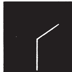
Diode paralleled by 680Ω
